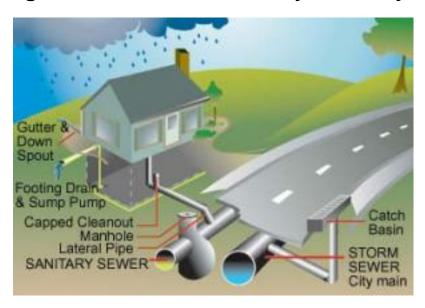
Illegal roof drains, sump pumps, and foundation drains connected to the City's sanitary sewer system sends groundwater to the sewer treatment plant, consuming expensive wastewater treatment capacity. Property owners need to disconnect these prohibited connections or be willing to pay for future treatment plant expansions.
