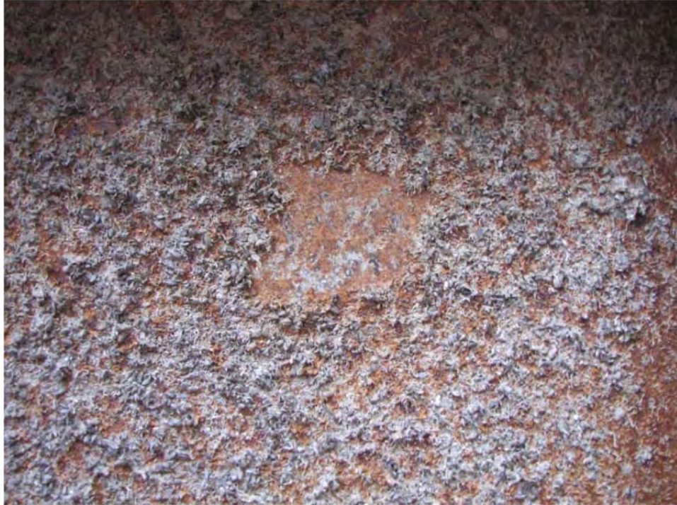
Photo 17. Bare spot is where the sample of the encrusting organisms was taken for microscope evaluation. No living organisms were found.
