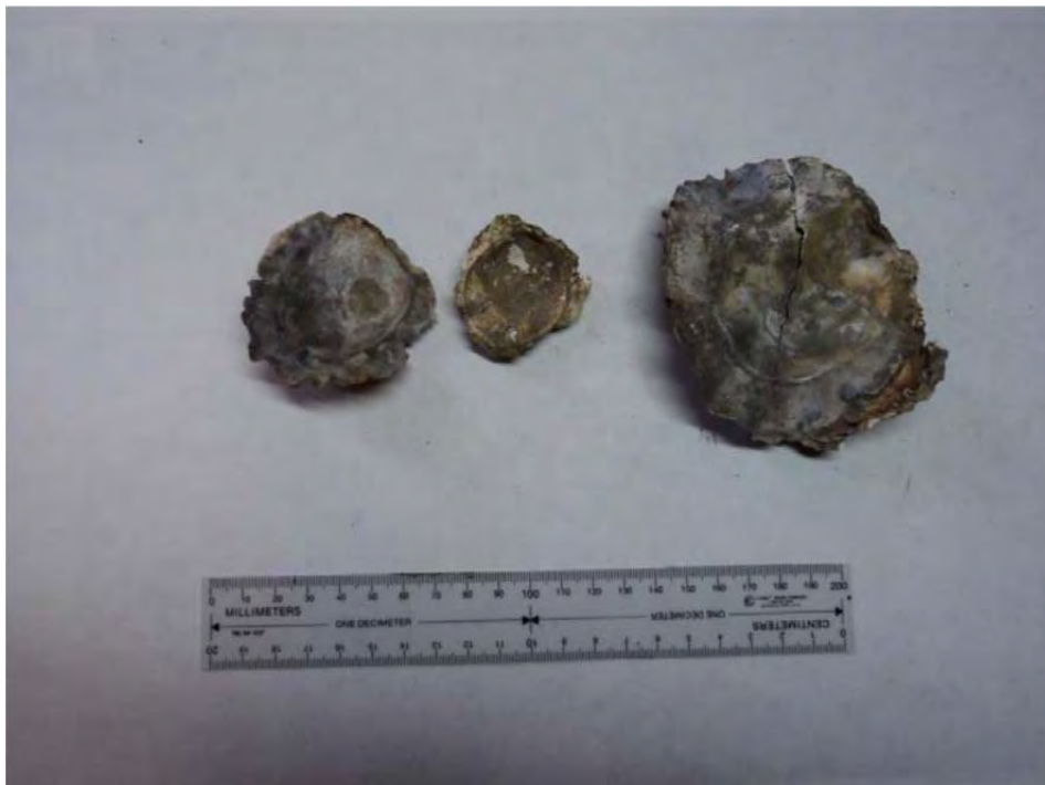
Photo 12. Right valves of oyster shells that have fallen from the legs. Oysters been dead for an extended period and shells are deteriorating.
