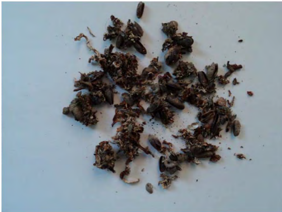
Photo 18. Dry, encrusted marine biota from the spud can sample scrape with barnacles, tube worms, mussels, and other marine debris. Dried fly larvae (maggots) were also in the material.
