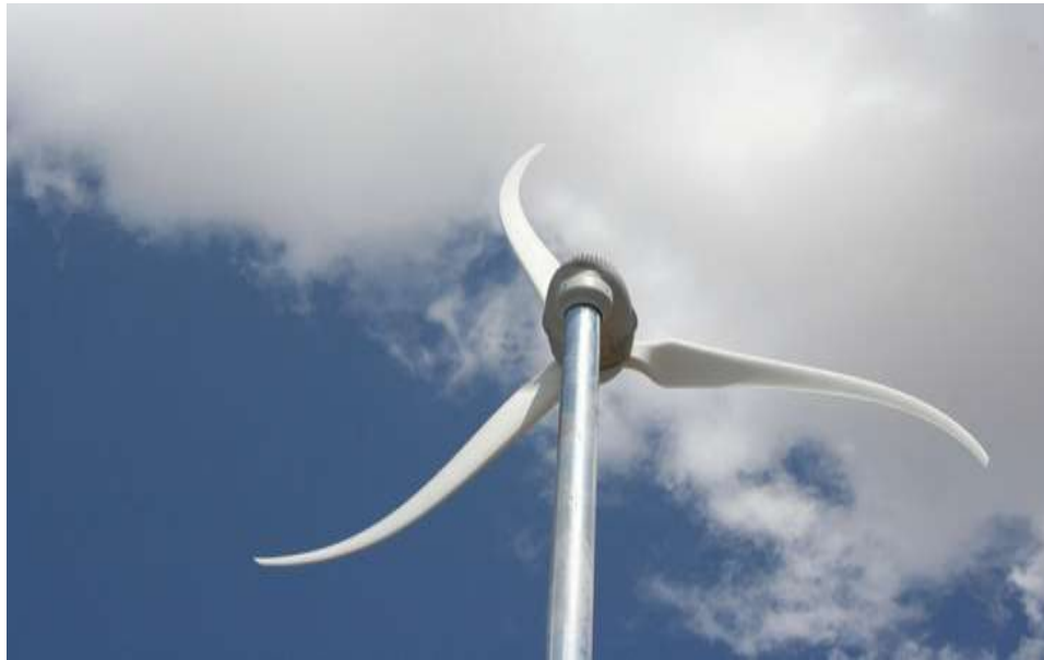
Figure 52 SkyStream 3.7 turbine (horizontal axis with curved blades)
