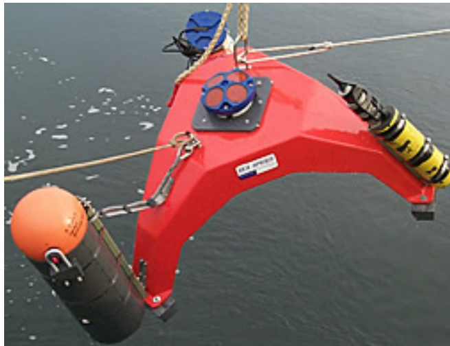
Figure 26: Oceanscience Sea Spider during deployment. Retrieved from http://www.oceanscience.com
