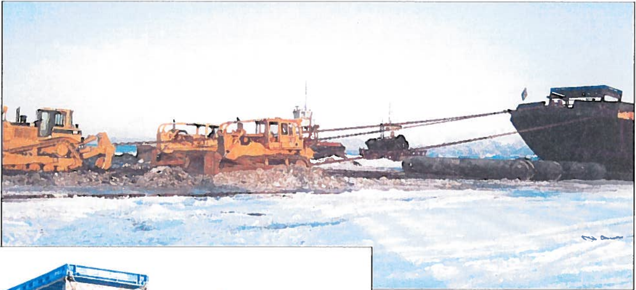
Cook Inlet Marine's Barge Lash 200 being hauled out onto the beach using massive inflatable bags, March 5, 2012
