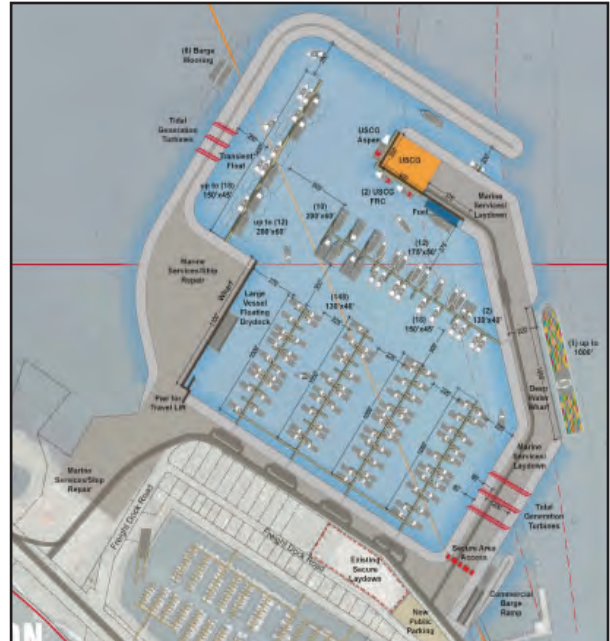
Port expansion adds a new basin with its own entrance adjacent to the existing Small Boat Harbor. It will relieve large vessel congestion in the small boat harbor, provide secure moorage compatible with the USCG’s assets and cargo areas..
