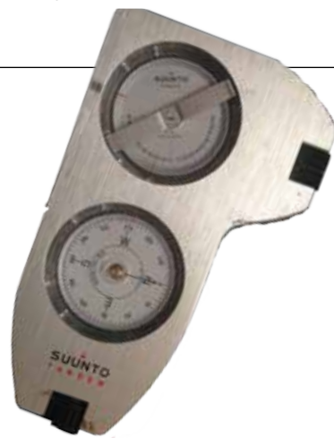
The Suunto Tandem is a commonly available clinometer suitable for trail assessment.
