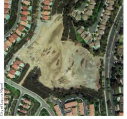
**Figure 7-1.** Aerial view of landslide triggered by El Nino winter storms of 1997-1998 in the city of Laguna Niguel. This slide occurred in an existing hillside development, within engineered slopes, destroying over a dozen homes.
