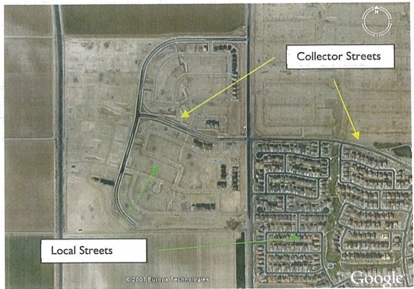
Figure 8: Collector streets and local streets being constructed at the same time.
