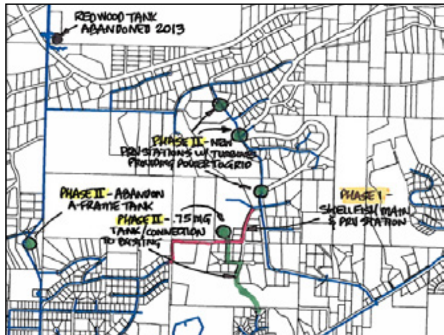
Phase 1, Shellfish Subdivision Main and PRV Station (indicated by red line) was completed in 2016. Phase 2 (green line) consists of installing an underground water storage tank and 2,000 linear feet of water main to increase water storage and distribution capabilities.
