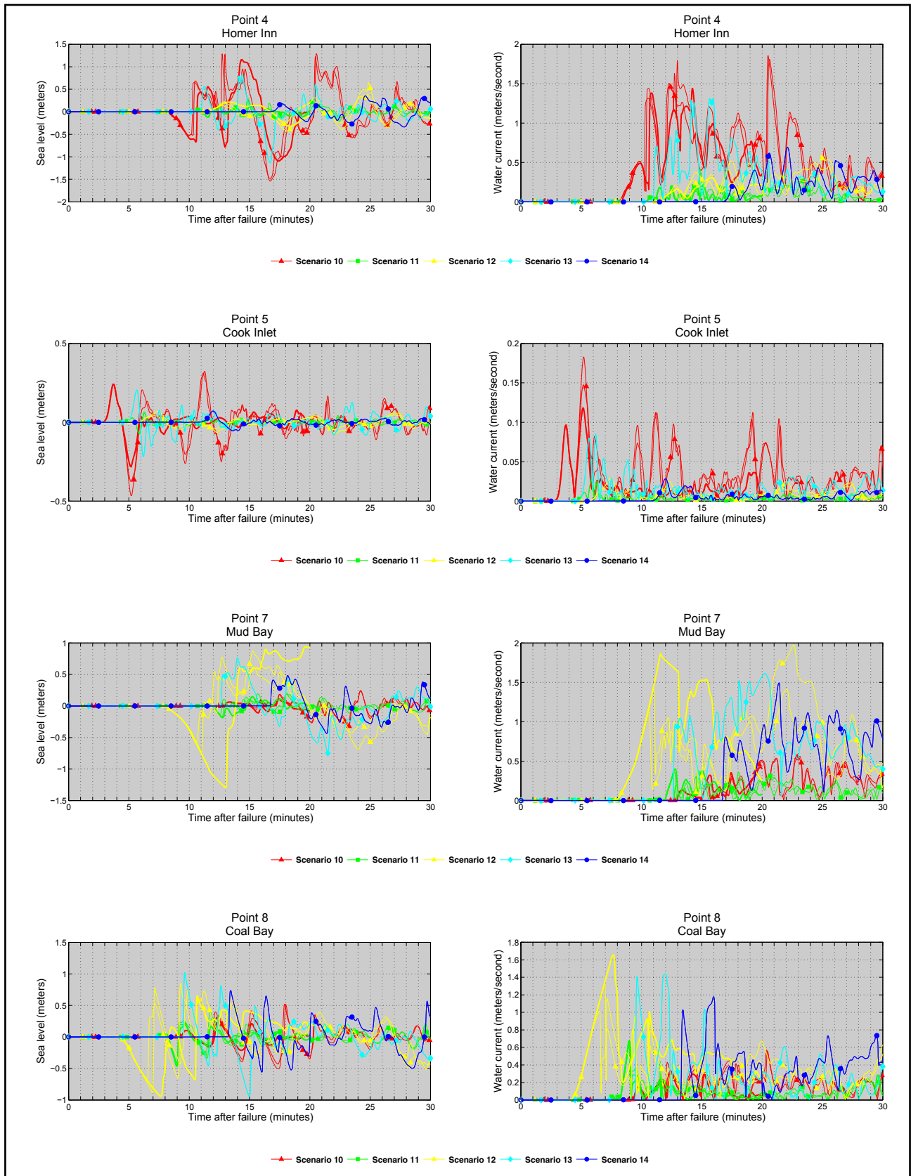
Figure A6. Time series of water level (left column) and velocity (right column) for landslide scenarios 10-14 at selected locations shown in figures A1 and A2.
