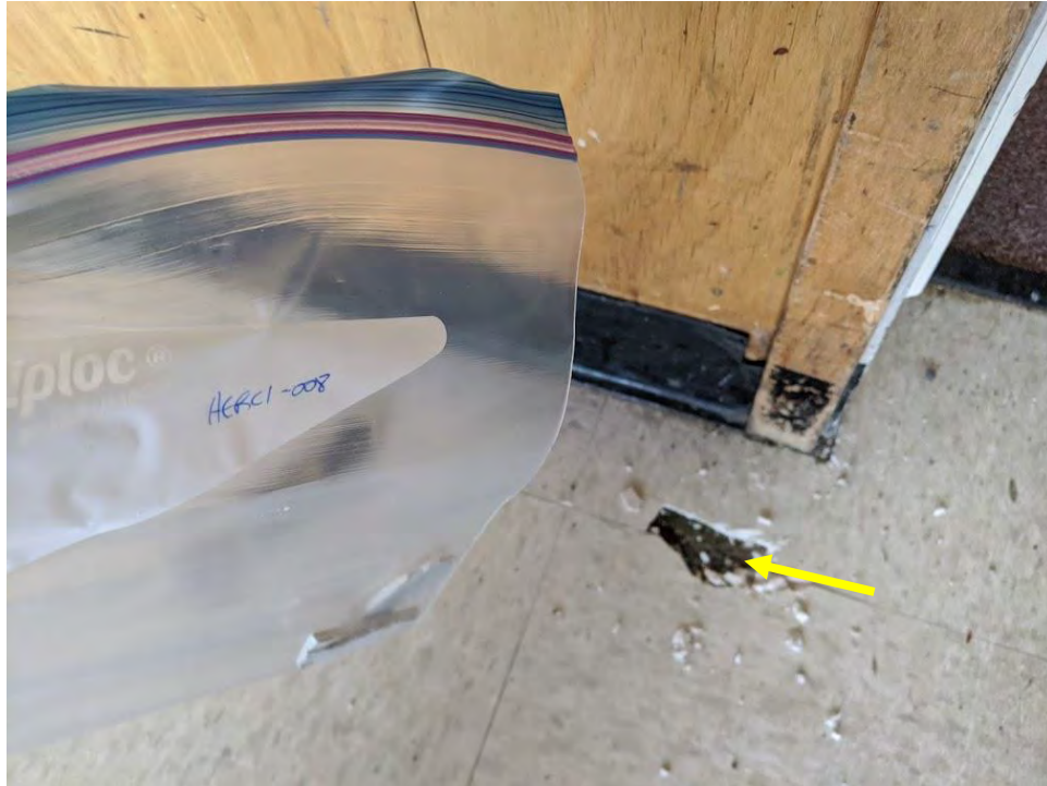
Photo 1: This photo shows sample location HERC 1-008 which is of ACM black mastic under the floor tile in room 107.
