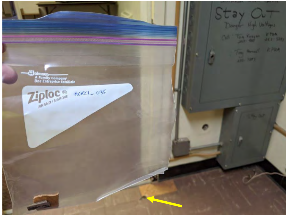
Photo 13: This photo shows sample location HERC 1-035 which is of ACM black mastic under the floor tile in the storage closet of the fan room.
