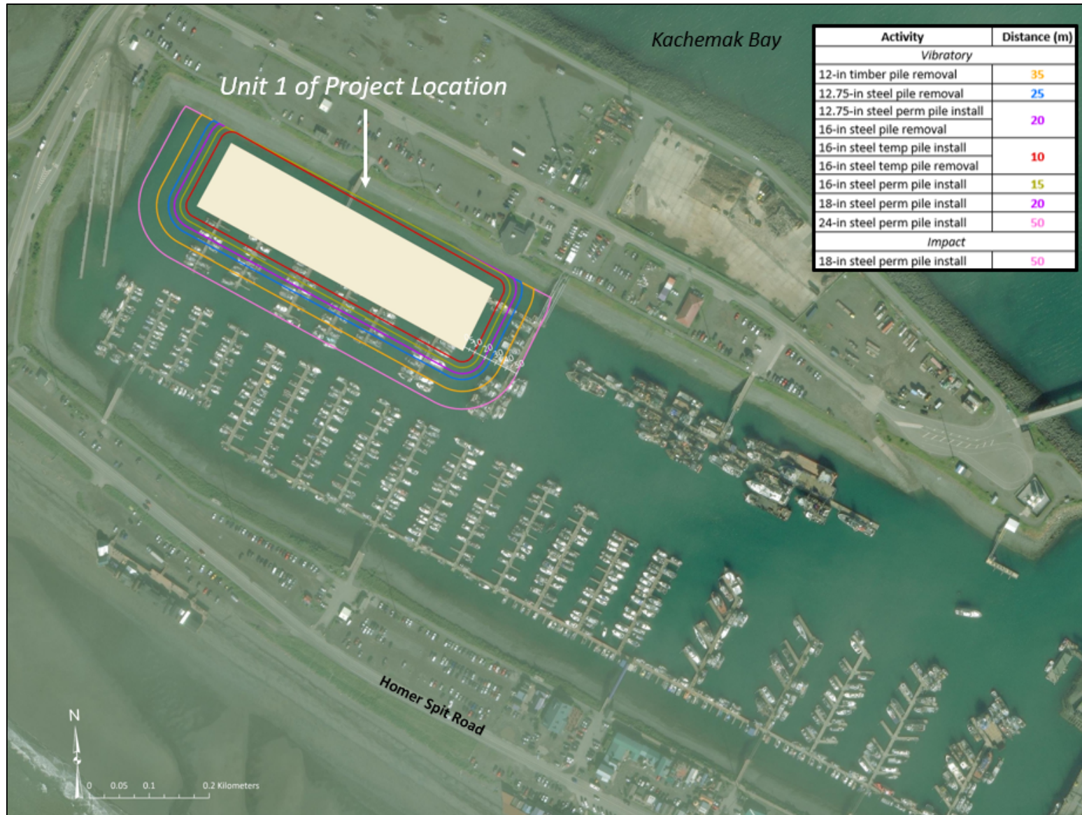
Figure 11. Homer Boat Harbor System 4 Float Replacement Project Unit 1 PW Shutdown Zones
