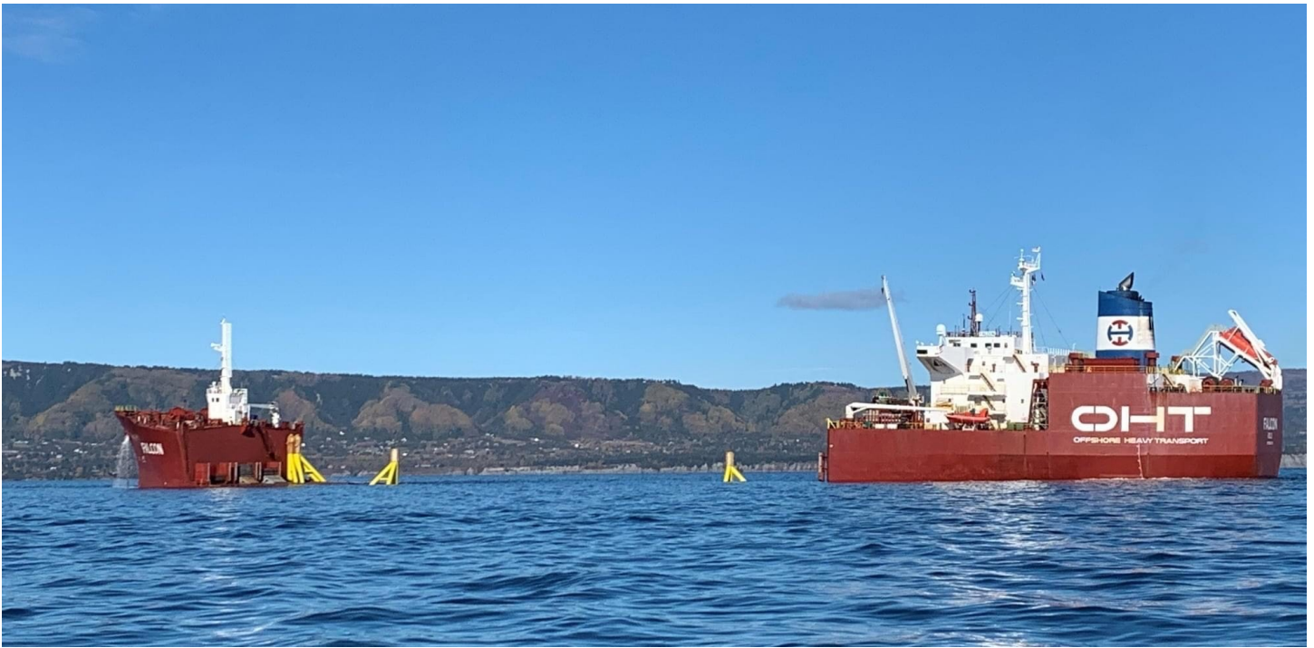
Ship decks intentionally submerged in preparation to load the drill rig Randolph Youst
