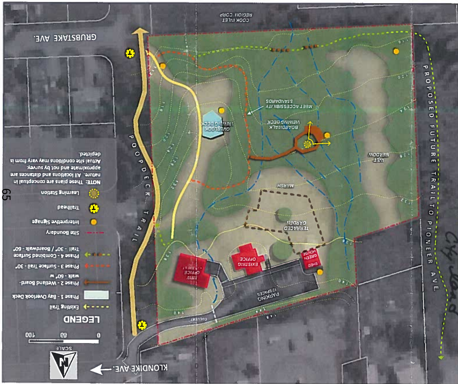
BOARDWALK SECTIONS: 60" Boardwalk over perennial and ephemeral wet areas. Tread 30" or more above grade will require guardrails. Construct with sustainable methods and materials.
