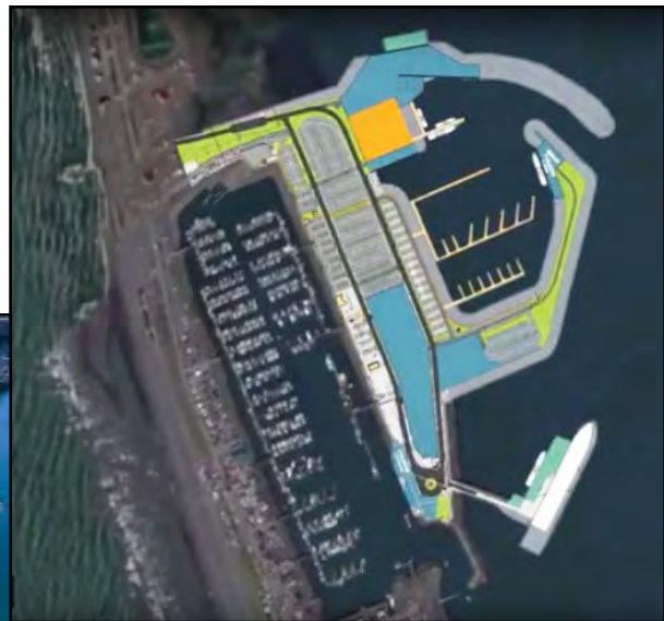
The large vessel port expansion adds a new basin with its own entrance adjacent to the existing Small Boat Harbor. It will relieve large vessel congestion in the small boat harbor and will provide secure moorage compatible with the USCG’s assets .
