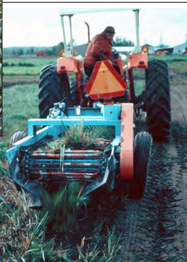
FIGURE a.12: A potato digger used to harvest Beach Wildrye at the Alaska Plant Materials Center
