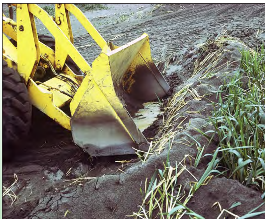
FIGURE a.11: Loader preparing to lift a natural stand of Beach Wildrye for sprig harvest
