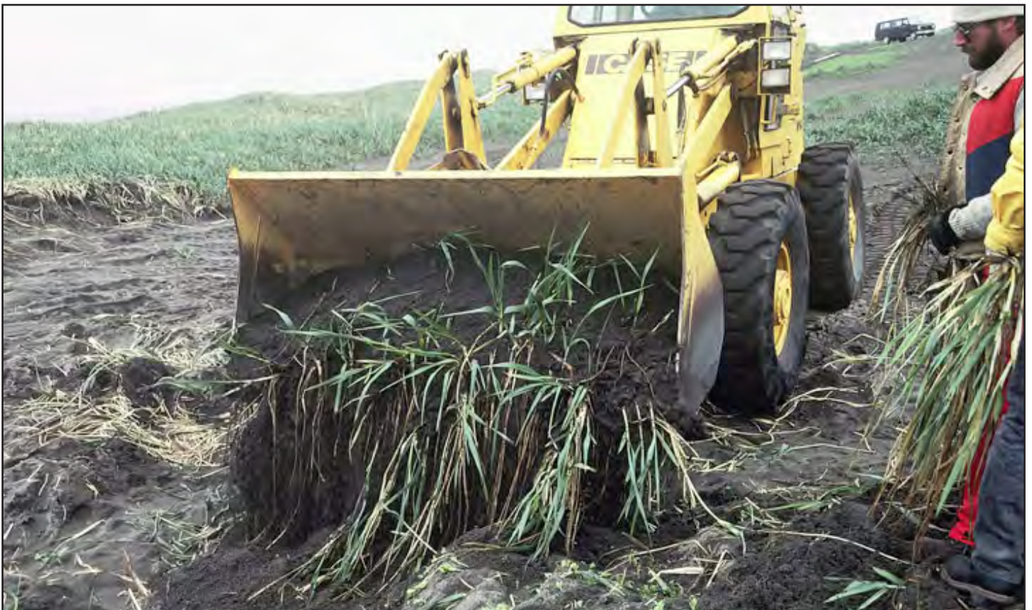
FIGURE a.10: Loader used to harvest sprigs
