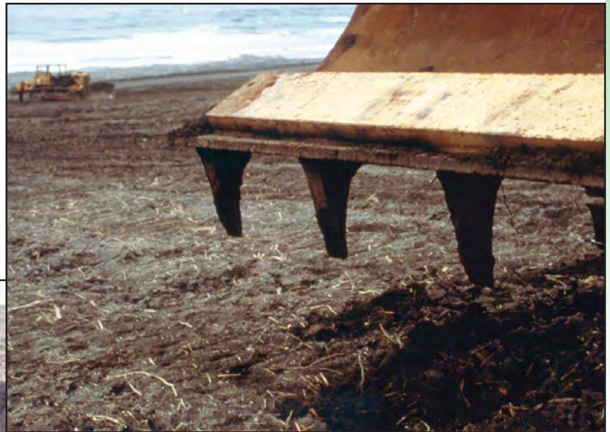
FIGURE a.13: Modified dozer blade with 'tiger teeth'
