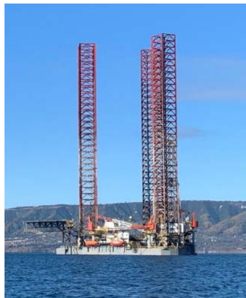
Jack-up drill rig Randolph Yost with its 400' legs fully elevated.
