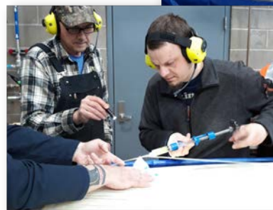
Left: Joe Young patching a single water filter membrane by injecting a silicon solution into the membrane. It's like giving someone an IV.
