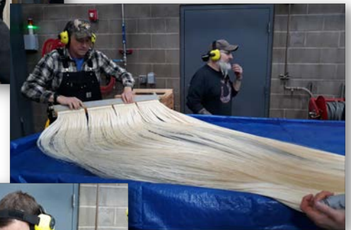
Left: Joe Young patching a single water filter membrane by injecting a silicon solution into the membrane. It's like giving someone an IV.
