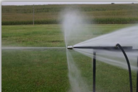
Jet angle on a Lance Nozzle.
