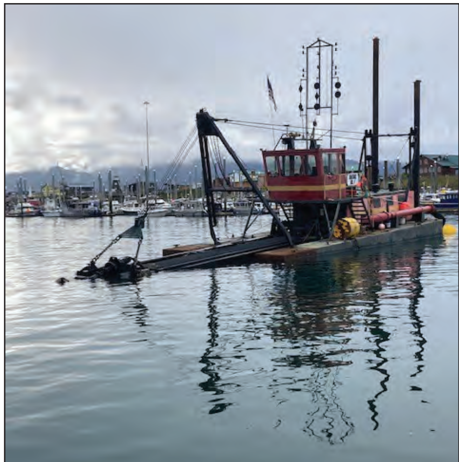
A dredge in Homer Harbor during the US Corps of Engineer’s annual dredging of the harbor’s navigable channel.
