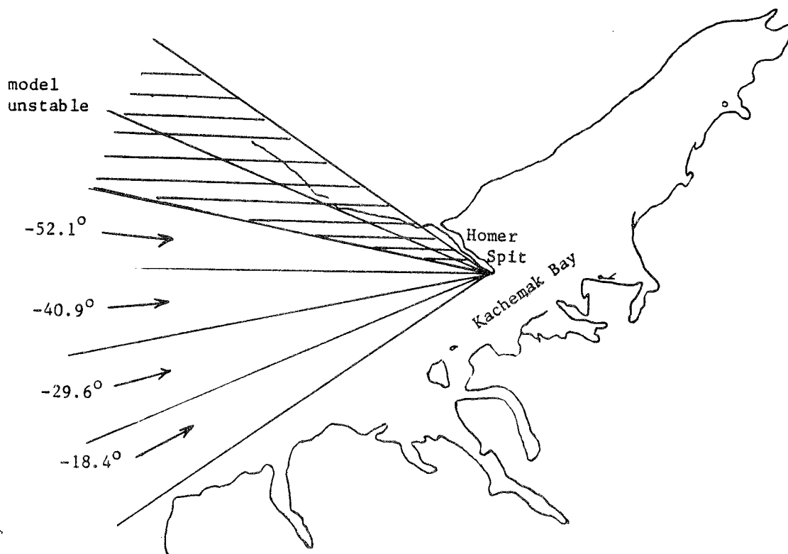
Figure B8. Wave direction bands relative to the transformation grid for time-history approach
