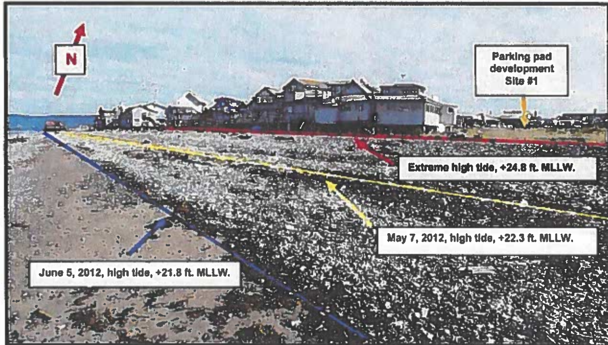
Figure 39. Parking pad development Site #1 on Homer Spit, Alaska in proximity to different tide levels.
