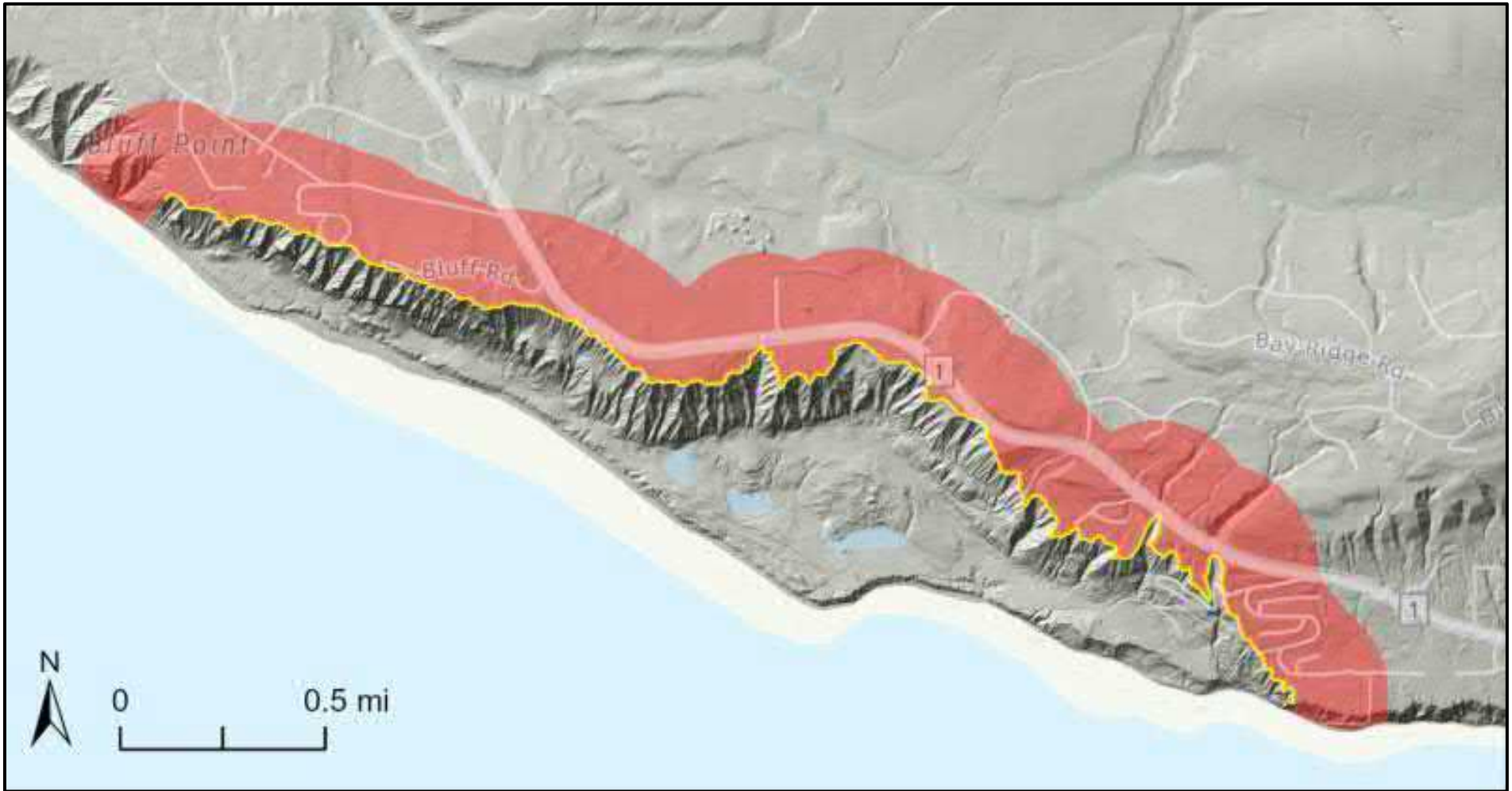
Deep-seated landslide susceptibility near the Bluff Point Landslide. Note that the landslide body (southwest of the yellow headscarp line) is also a landslide deposit and is highly susceptible to repeated failure.
