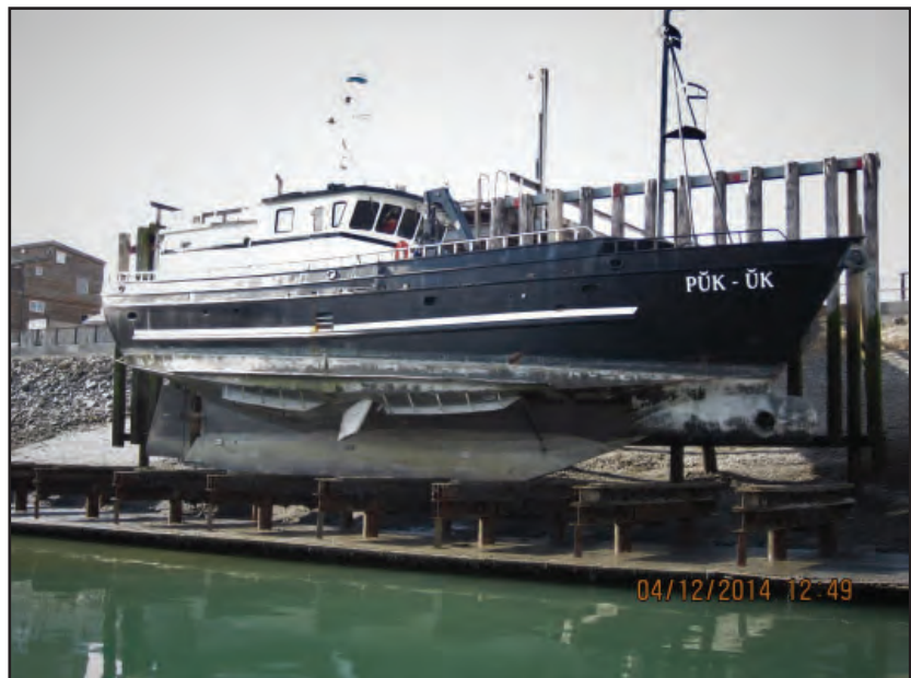
A marine vessel utilizing Homer Harbor’s steel grid for repairs.
