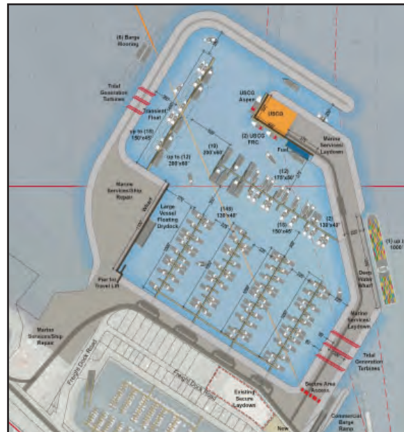
Port expansion adds a new basin with its own entrance adjacent to the existing Small Boat Harbor. It will relieve large vessel congestion in the small boat harbor as shown below..
