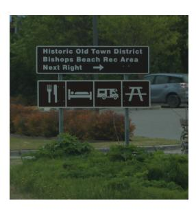
The Directional - Road (ADOT&PF) is used to direct vehicular traffic. These require ADOT&PF permitting and design and construction need to meet ADOT&PF standards.
