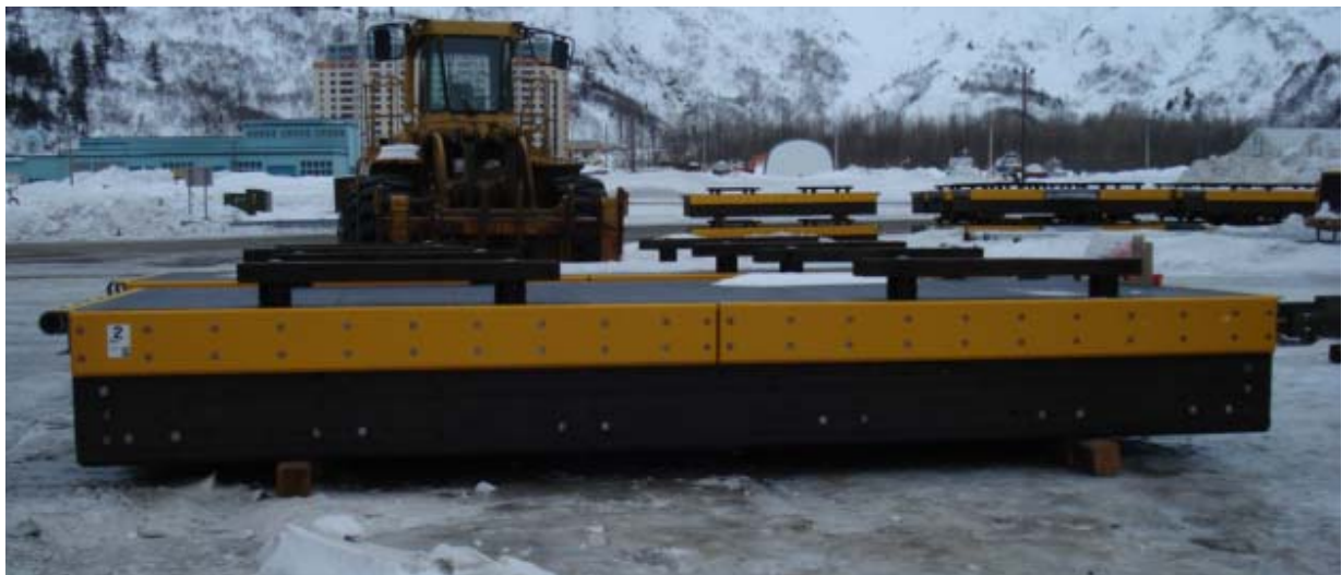
Figure 3-1: Timber Launch Ramp Float Unit
