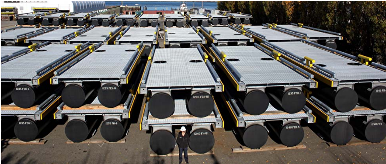
Figure 3-3: Modular Pipe Float Units
