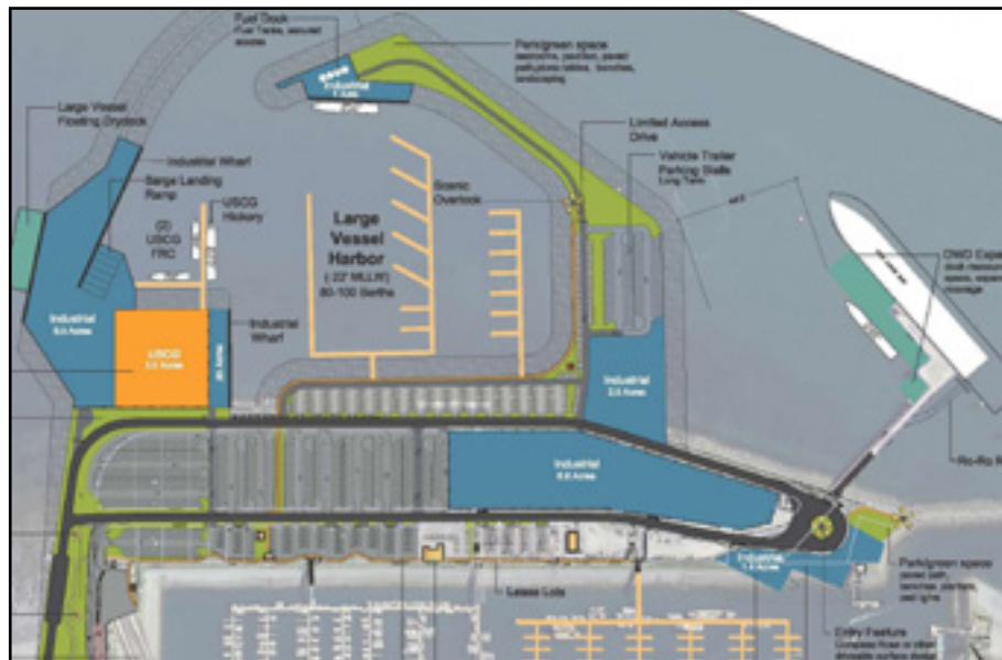
This large vessel harbor design adds a new basin with its own entrance adjacent to the existing Small Boat Harbor. It provides secure, larger-sized moorage compatible with the USCG's new line of fast response cutters .
