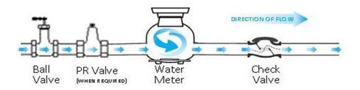
Meter shall be installed in a horizontal, upright postion.
